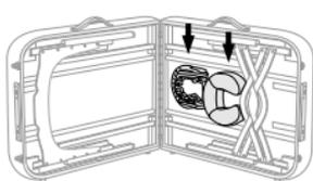
**2** Release the handle and extend the dowels outward. Lock the handle after the platform is set to the desired level.
